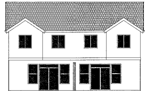
REAR ELEVATION SCALE 1/8"=1'-0"
