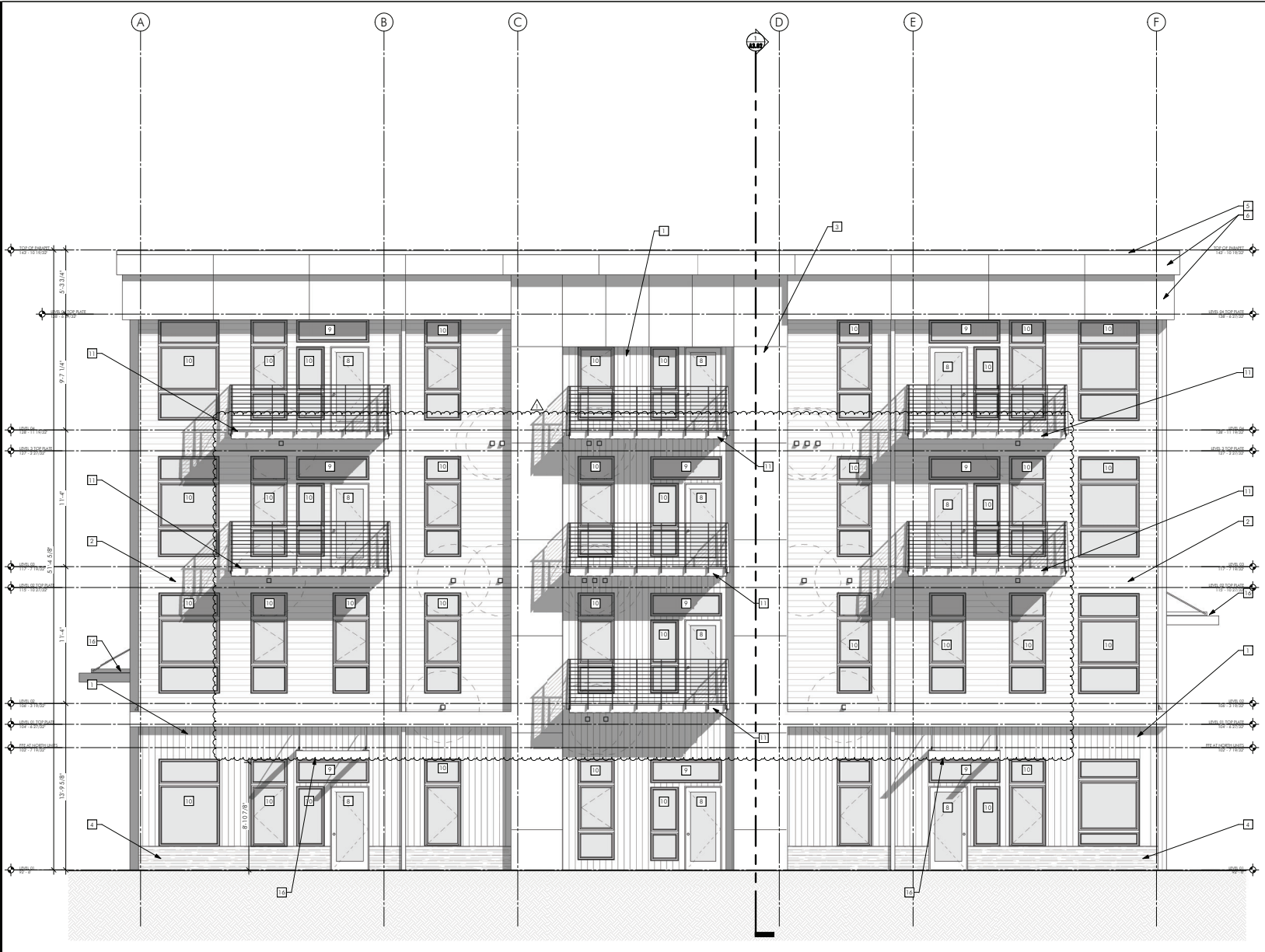
BUILDING B - SOUTH ELEVATION 1/4" = 1'-0"
